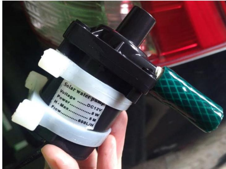
Gambar 34. *Solar Water Pump* 8 Watt 12 V
